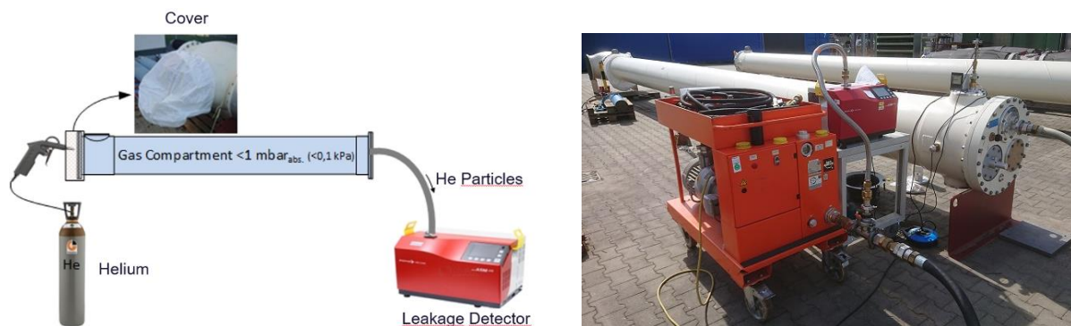
Figure 9 – Principle and test arrangement of the vacuum method
