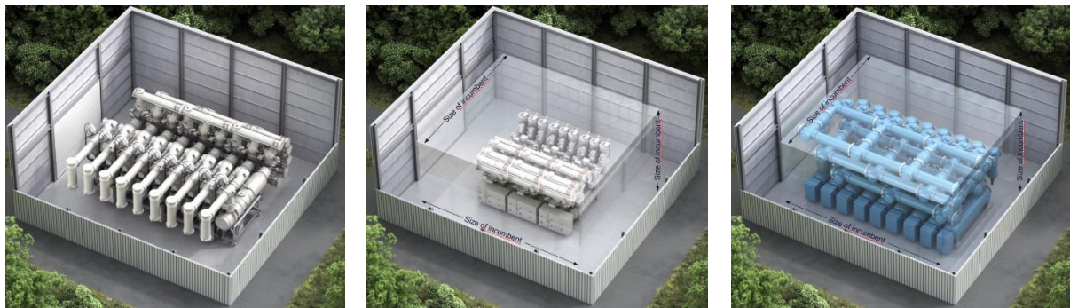
Figure 3 – Size comparison: previous SF 6 generation, current SF 6 generation, new clean air
