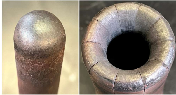
Figure 3: After complete L75 & T100a test sequence - Arcing contacts
