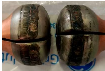
Figure 10. Wear while BTCS test - C4FN/ O 2 / CO 2 (to the left) & SF 6 (to the right)
