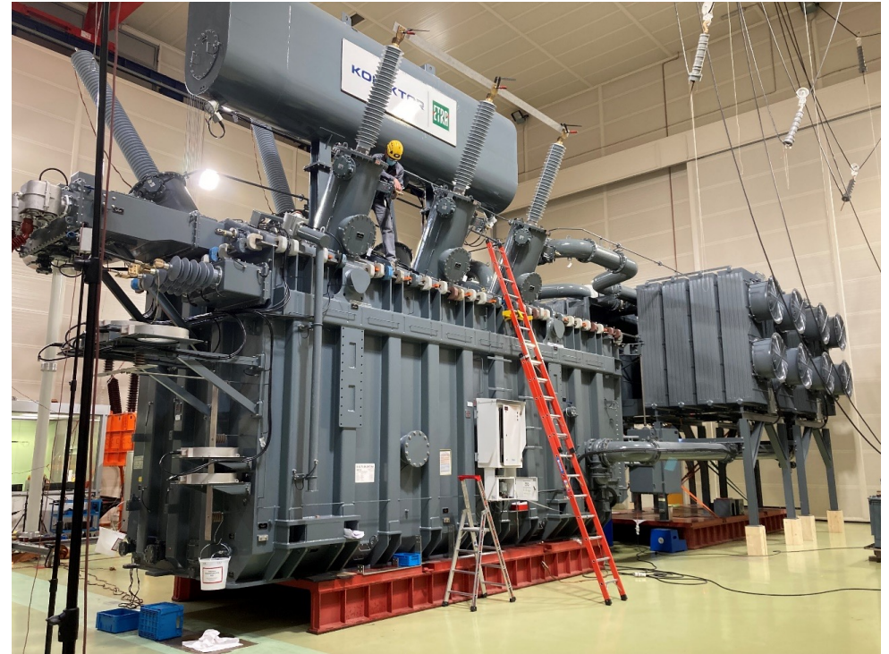
2022, line end tapchangers in-tank, 3-column
