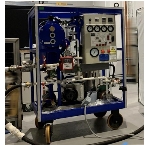
Oil processing unit (available at the UoM lab)
