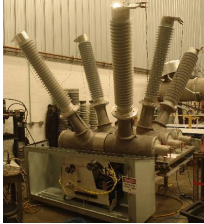
Figure 5: Dead tank 145g 3 during mechanical endurance test.
