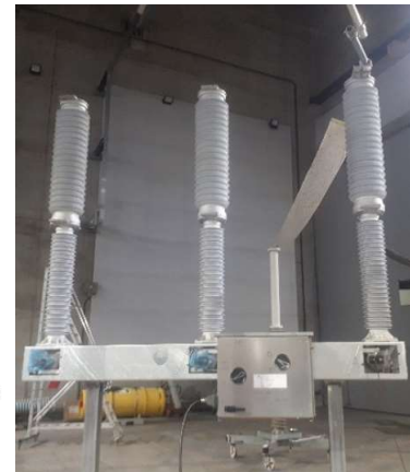
Figure 5: Results of TD2 & TD3 at 145 kV and picture of the 145 kV LT circuit breaker (C 4 FN based gas mixture)
