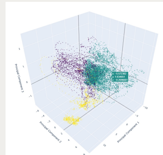
Figure 5 – Principal component space of PMU voltage measurements - clustered via k-means clustering
