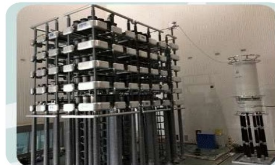
Figure 9: 500kV HVDC Breaker Type Test
