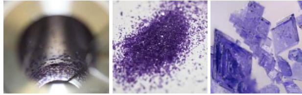
Figure 7: Crystals in the autoclave and microscopic view
