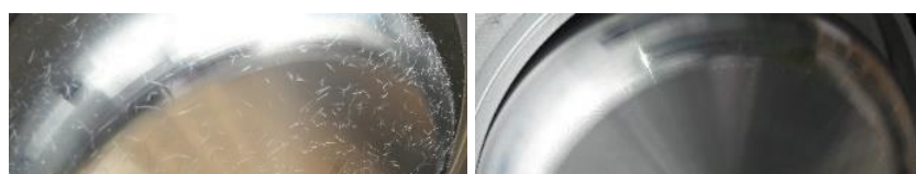
Figure 9: Amide type crystals in GC4 before (left) and after (right) sublimation
