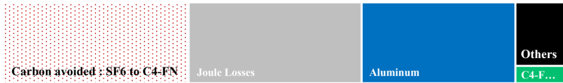
Figure 3 - Carbon origins for a 145kV C4-FN mixture GIS (-33% vs SF 6 version)
