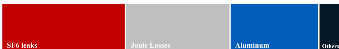
Figure 2 - Carbon origins for a 145kV SF 6 GIS (+50% vs C4-FN mixture version)
