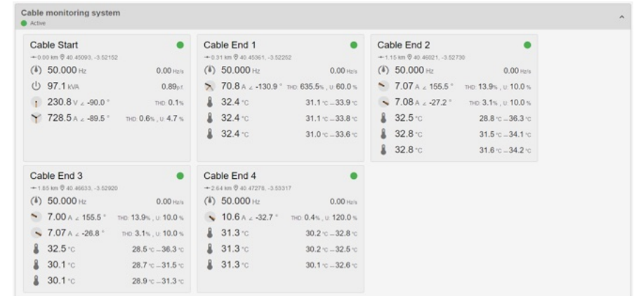
Dashboard of measurements, grouped by physical location
