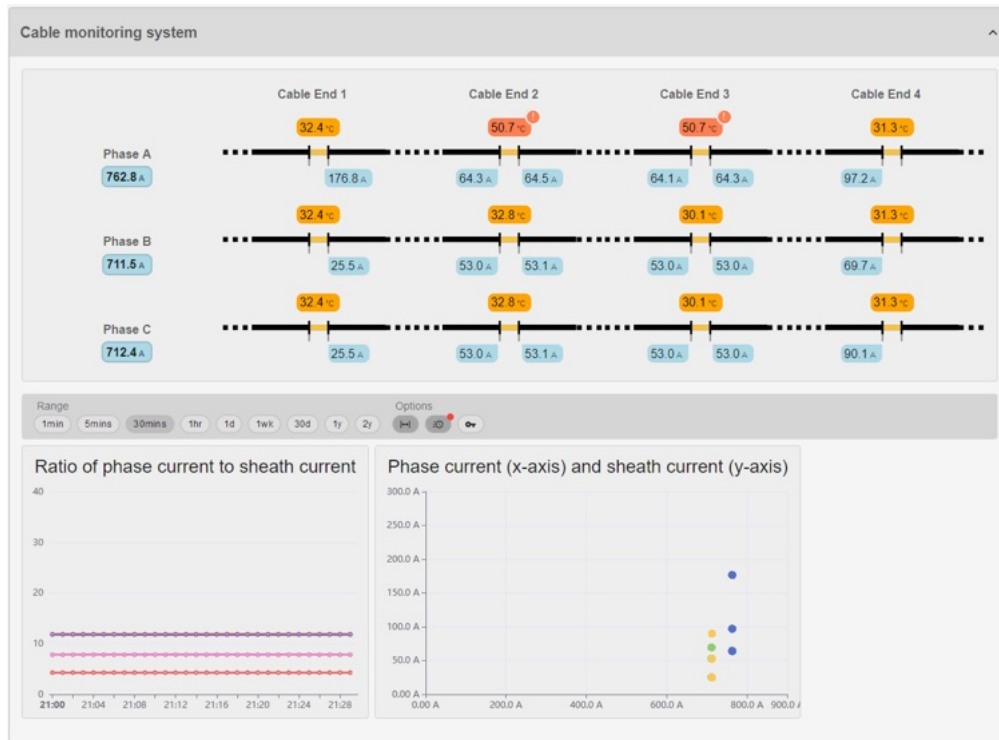
Cable health monitoring dashboard
