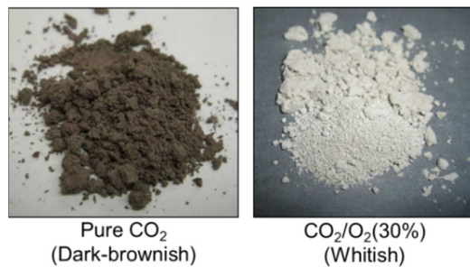
Figure 6: Solid by-products after arcing in pure CO 2 gas and CO 2 /O 2 gas mixture after 1,900 kJ accumulative interruptions.
