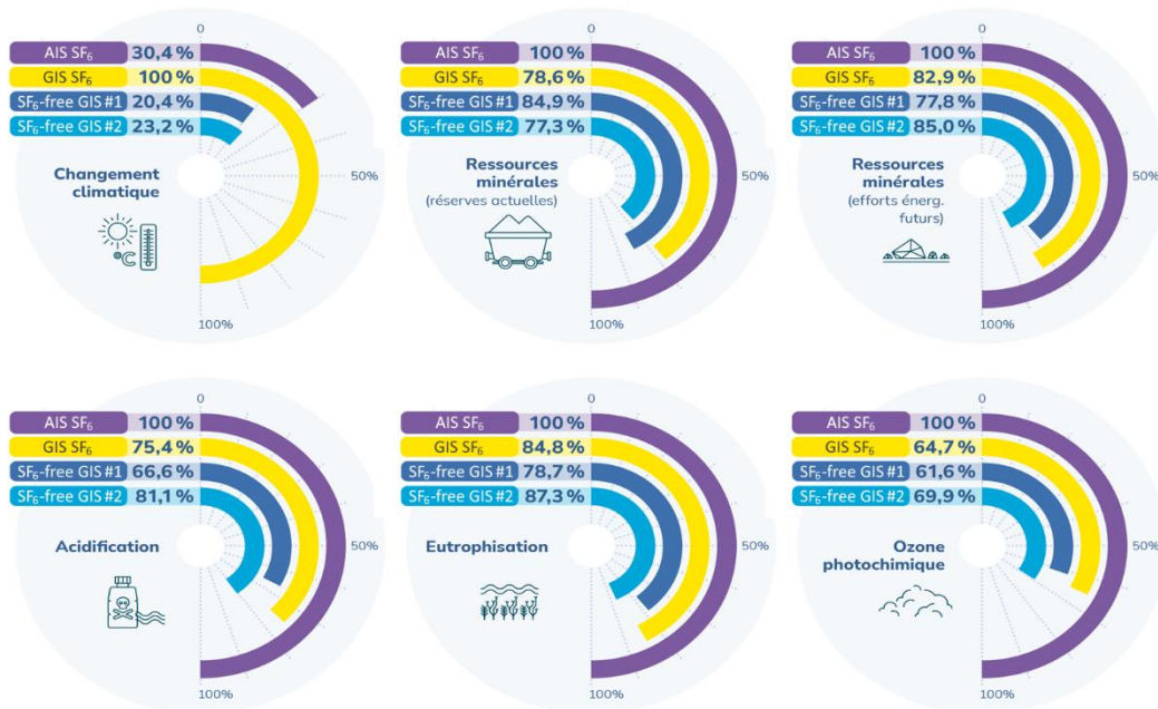
Figure 2 - LCA indicators retained by RTE for the comparison of 63 kV substations (different types and technologies)
