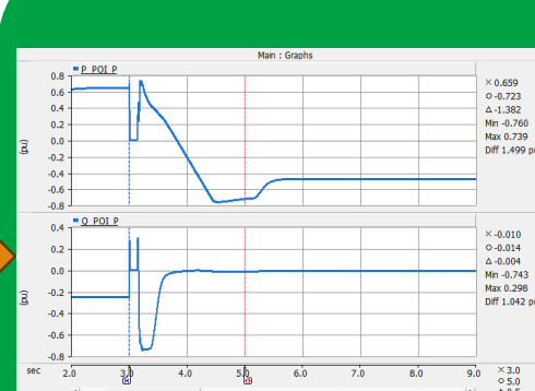
After the fault reactive power changed to zero due to current limitations.
