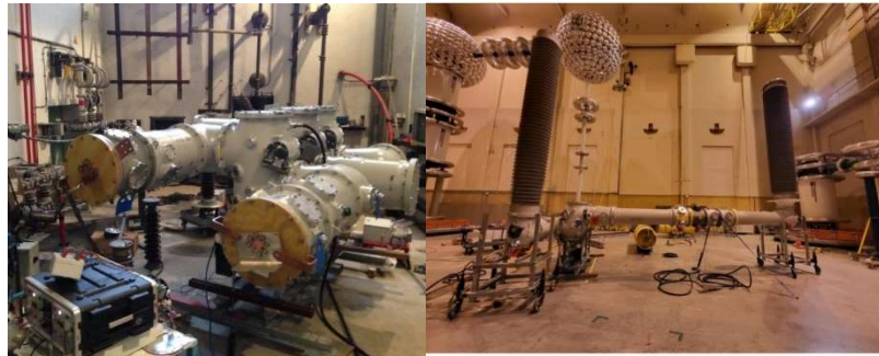
Figure 2 - Dual-gas three-phase disconnector arrangement during a type test campaign with SF 6 and C4-FN gas mixture, during power test (left) and during dielectric condition check (right)
