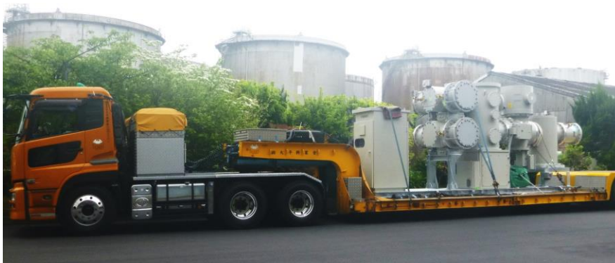
Figure 5: Transportation tests of the GIS.
