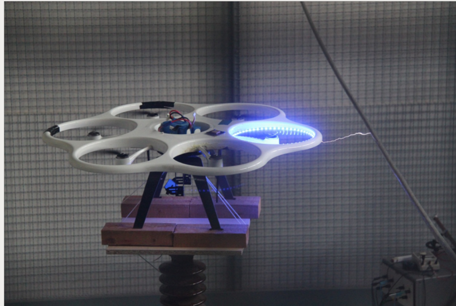
High voltage AC-test of a multicopter with a pre-discharge between phase conductor and multicopter housing
