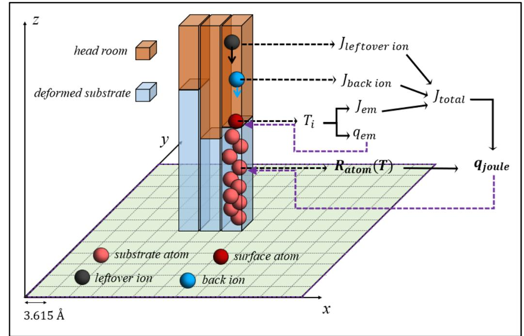
➤ MD simulation model of an individual cathode spot.
