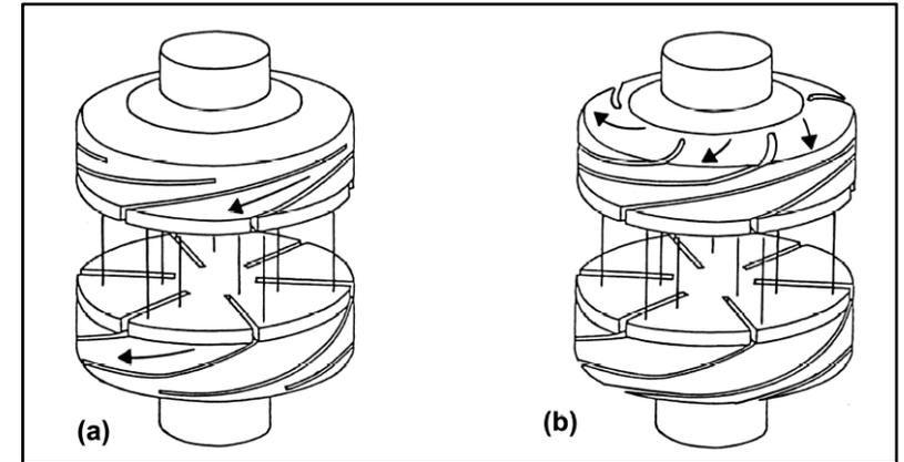
➤ Up: Structure of TMF contact and AMF contact.
