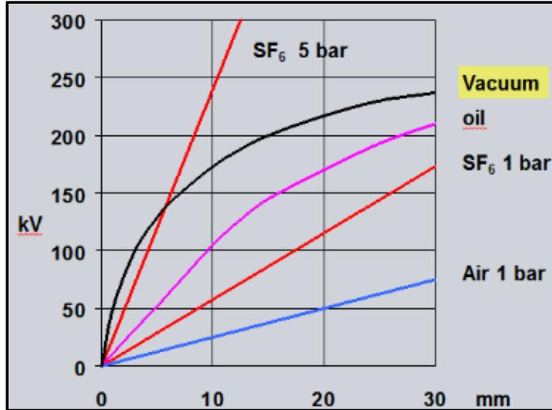
SF<sub>6</sub> gap: breakdown strength ~ gap length
