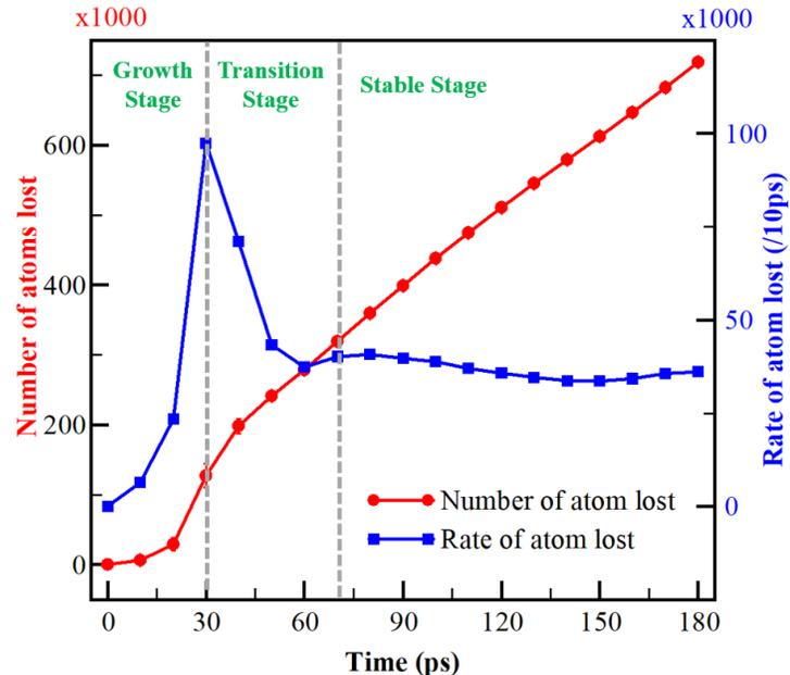
➤ Evolution of lost atom number and lost rate in the central position of a cathode spot.
