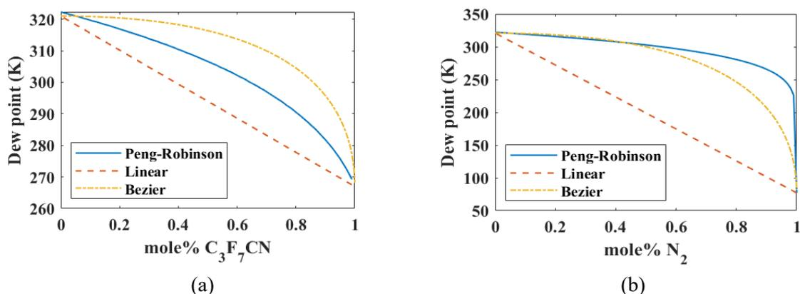
Figure 1. Comparison between dew point estimation methods (Bezier, linear) with calculated by Peng-Robinson Equation of State values [9], (a) – C<sub>3</sub>F<sub>7</sub>CN and C<sub>6</sub>F<sub>12</sub>O mixture with boiling point difference of 1.2 °C (b) – C<sub>6</sub>F<sub>12</sub>O and N<sub>2</sub> mixture with boiling point difference of 4.16 °C.
