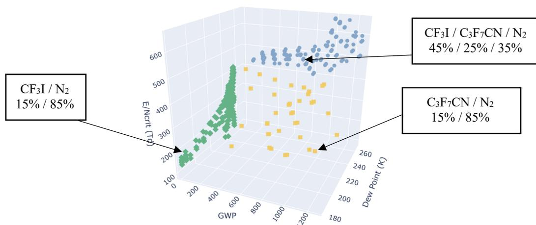
Figure 7. Pareto optimal solutions after 100 iterations: blue circle –  $(E/N)_{crit} > 400$  Td and boiling point  $> 255$  K; green diamond – GWP  $< 100$ ; and yellow square – other gases.
