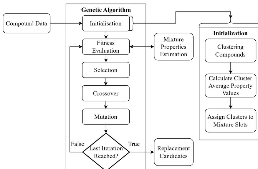
Figure 2. Mixture evolution program flowchart
