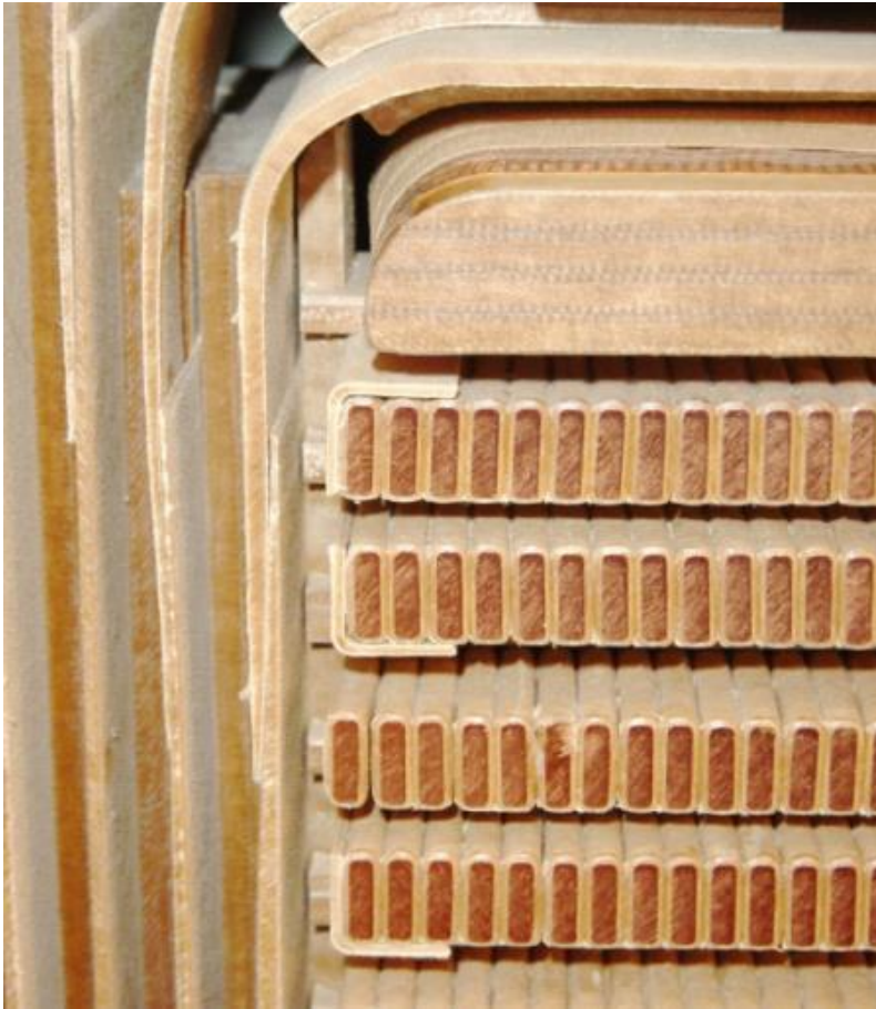
Cross-sectional view of 400 kV transformer end insulation*
