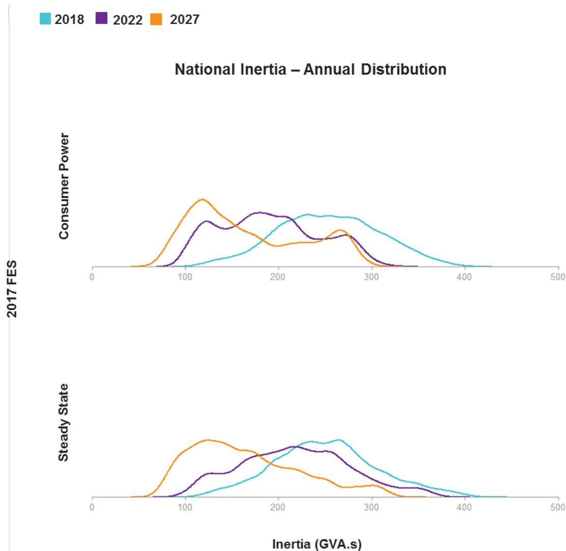
**Operating with low system inertia:** RoCoF relay changes and predicted reduction in synchronous generation resulting in reduced levels of system inertia (*unconstrained system*)
