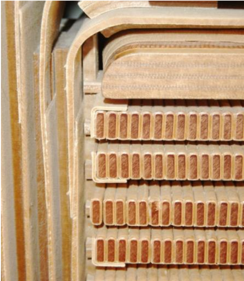
Cross-sectional view of 400 kV transformer end insulation*
